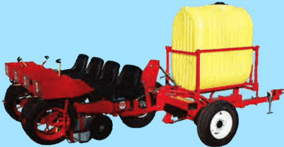
Model 803 2 1000 - Two row with NEW 803 heavy duty trailer. Shown with upright 300 Ga. tank, telescoping tongue, 4x7 toolbar and two Model 1000 units. Options: cushion seats, double disc poly shoes, rubber packing wheels and 7:60 x 15 tires.
