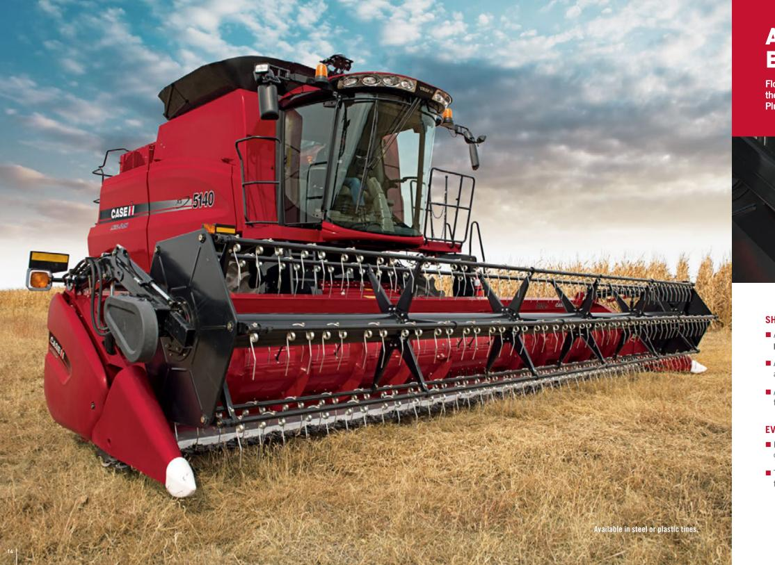
Float over challenging ground contours with the 3020 series flex auger head. Designed to limit grain loss and increase harvest efficiency, the flex head guarantees even crop feeding with its seamless transition from the cutterbar to the standard stainless-steel augur floor. Plus, between the optional TerraFlex<sup>™</sup> suspension system and rigid cutterbar mode, you'll have the ability to harvest all crop types.
