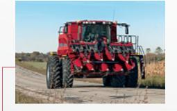
Case IH offers folding corn heads in 8-row and 12-row configurations. Capable of folding into transport mode in less than a minute, folding heads dramatically improving transport efficiency, and, ultimately, field productivity.
