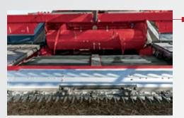
A seed saver channel along the bottom of the draper belt smoothly pulls grain into the combine, saving up to three percent more grain so no seed is left behind.
