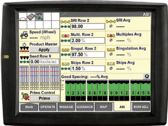
The AFS Pro 700 display runs six screens on a single monitor that allow you to control key machine functions.
