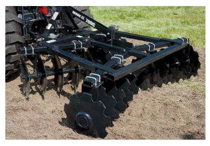
**The Work EZ disk harrow** from Case IH offers a cutting width of 70 in. for tractors up to 70 hp.
