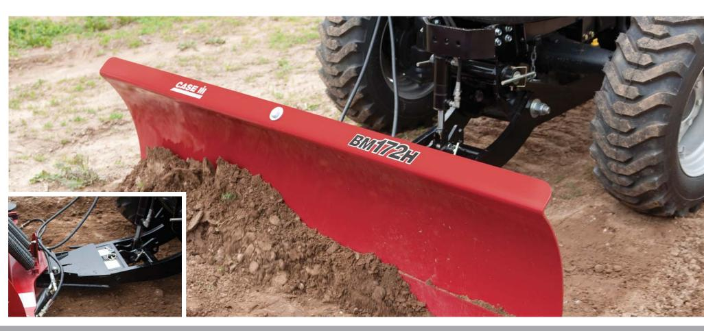
Case IH **Quick-Attach front blades** bolt on for long life and easy maintenance, and are easily attached and removed without tools. The **durable cutting edge** on Case IH Quick-Attach front blades is made of heat-treated, high-carbon steel that's reversible and replaceable. The **blade angle adjusts** from 0 to 30 degrees, while its up-front position makes it easy to see and manage your load.
