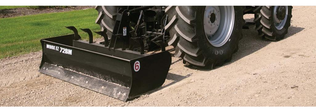
**Work EZ box blades** from Case IH include heat-treated, easily adjustable scarifier shanks with replaceable tips to rip through hard-packed soils.
