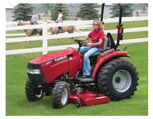
Routine maintenance is a snap on Case IH MW mid-mount mowers, because spindles can be greased from the top of the mower deck without removing the shields.
