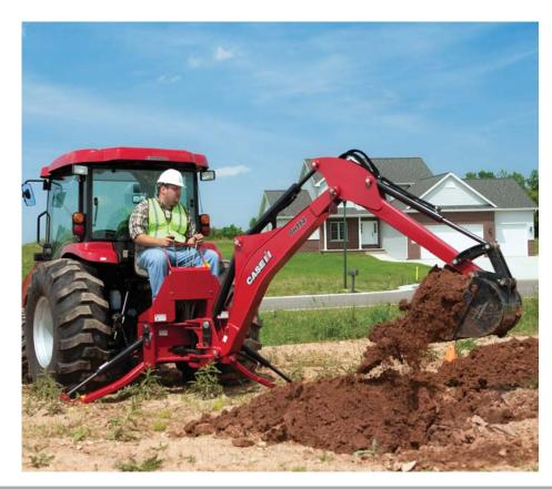
On **Case IH utility backhoes**, all controls are mounted in a low-profile console that doesn't block your view.
