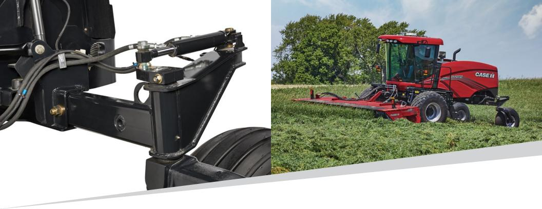
The rear steering manifold and steering cylinder enhance control and stability by
