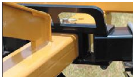
Easy-to-grasp handle for simple gang adjustment
