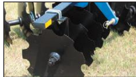
Notched discs for maximum cutting action
