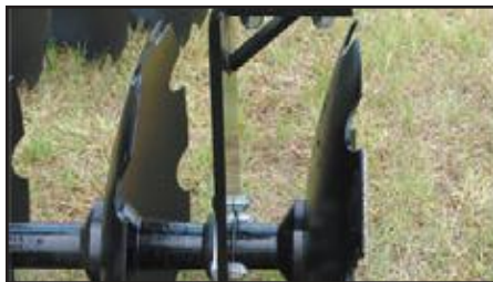
Bearing hangers reinforced with gussets
