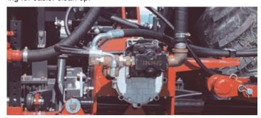
A Cat 4 driveline is standard equipment on the DB150, allowing for easy unit hook-up. The speed increaser and hydraulic pump are mounted to the frame for a secure mount and easy access to component parts. A heavy duty ball valve separates the hydraulic reservoir from the hydraulic pump, motor, and hoses and can be closed to reduce oil loss during maintenance and repair. The driveline is fully shielded for enhanced safety.
