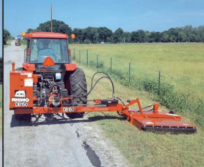
The DB150 can be retracted to a width of 119" for easy transport on narrow roads and through narrow gates. The operating range of the head is 85° up and 90° down to handle many different applications. The transport-locking arm can be attached easily to lock the head in transport position for enhanced safety during transport. Unit hook-up and storage is made easier by the standard support stand.
