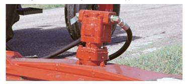
The hydraulic motor of the DB150 mounts to the frame, not the deck, to help reduce downtime and repair costs. The gearbox mount access hole allows for easy access to the spindle housing grease fitting. The clean deck design of the DB150 increases the life of the unit by allowing for easier clean-up.
