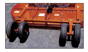
An optional auxiliary wheel spindle kit is available for both the TW120 and TW144 pull-type units. The kit easily bolts into the axle arm beam for those applications where dual wheels are needed for added flotation and stability.
