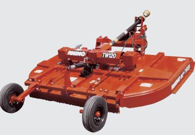
A spring shock absorber is available as optional equipment for the pull-type TW120 and TW144. The springs help cushion the shock loads that the deck will encounter when operating in rough terrain. Standard hydraulic control spacers are used with the available hydraulic cylinder to set the cutting height on pull-type units.
