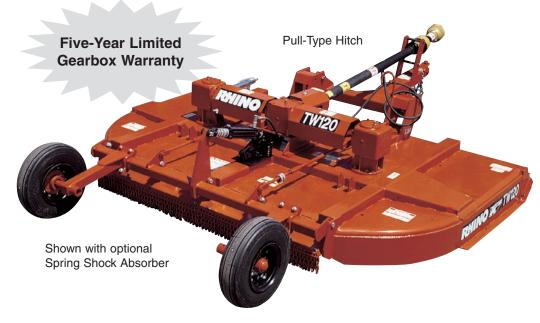
The TW120 cuts a 120" swath of material. The center gearbox, rated at 120 HP, transfers power to the 100 HP outboard gearboxes. Torque dampeners on both sides of the center gearbox help minimize driveline and gearbox damage caused from sudden shockloads. Massive 2-3/8" diameter output shafts in the outboard gearboxes help provide optimum service. The pulltype unit requires a 50 HP (min.) tractor and the lift-type unit requires a 60 HP (min.) tractor (with adequate front weights).
